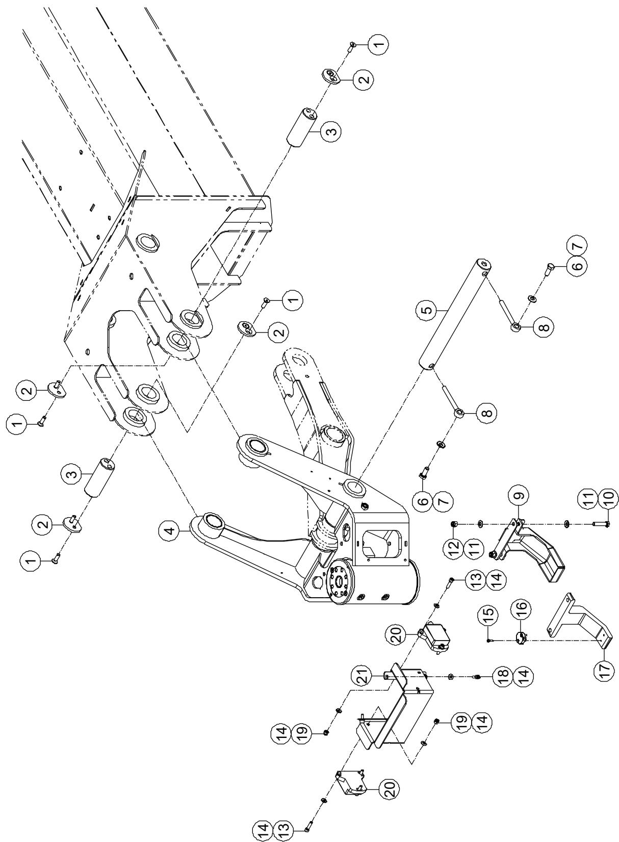
**3-33 Rotate Cylinder Assembly Installations**
