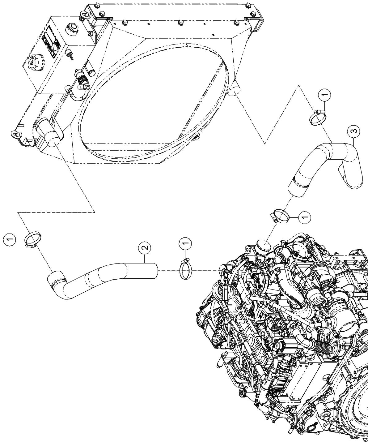
**2-18 Engine Cooling System Installations 2**
