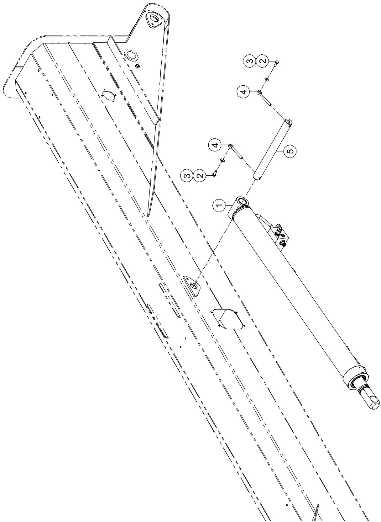
**3-31 Leveling Cylinder Assembly Installations**
